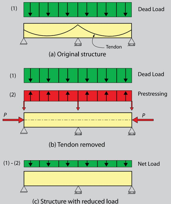
Fig. 4: Simple load balancing
