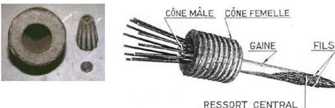
Fig. 3: Freyssinet's early anchorage device: (a) photo of anchorage device; and (b) diagram of anchorage assembly
