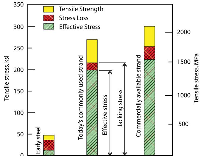
Fig. 2: Comparison of steel strengths and prestress losses for steel used in early attempts at prestressing and those currently available
