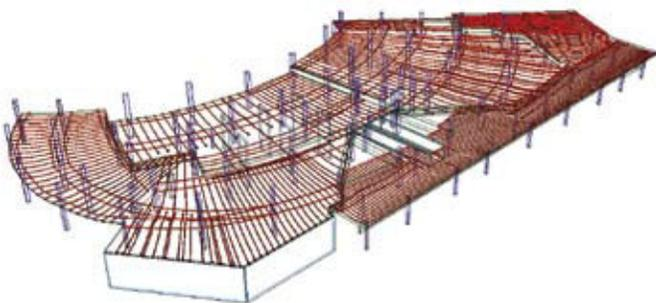
**Fig. 5: Post-tensioned podium slab with irregular support layout and multiple steps on the top and bottom of the slab**
