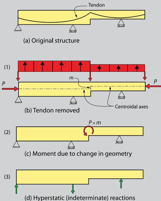
**Fig. 6: Extended load balancing**
